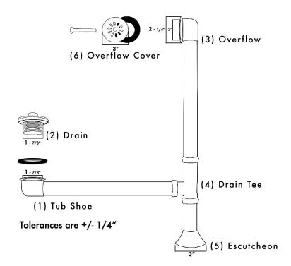
Its always advised to place plumber's tape onto any threads during any plumbing installation.
